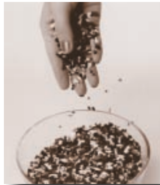
Granulated recycled ABS resin.
